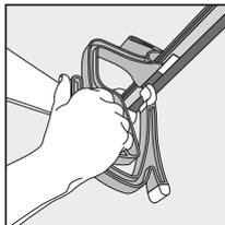
**Put the Side Clamp and Foam Rail into place.**
