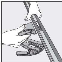
Attach the Side Clamp to the Foam Rail by pressing the thumb release. Place the Foam Rail into Side Clamp's rail catch and release thumb pressure. To center the Side Clamp on the rail, place at the Foam Rail label.
