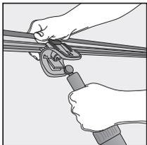
Snap the Clip on the ball at the top of the ZipWall® pole. Now, with the Foam Rail attached to the pole, raise it into place, pressing the barrier against the ceiling.
