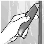
4. Carefully unzip the zipper completely. Then, using the opening as a guide, cut the plastic to make the doorway.
