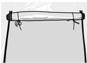
6. For a wide doorway, install another zipper on the plastic as far away from the first zipper as you want the opening to be. After both zippers are installed and opened, use the enclosed string to tie up the loose plastic at the top of the doorway.
