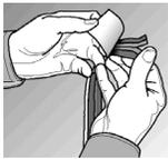
2. Be sure the plastic or barrier material is clean. Hold the zipper up to the plastic to determine where you want it. **The pulls should be at the bottom!** Be sure the entire length of the zipper has plastic to stick to. Then start to peel the paper from the back of the zipper at the top and begin to press the zipper onto the plastic.
