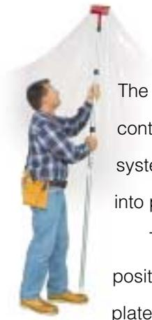
The **ZipWall® barrier system** is an easy way to contain an entire work area in minutes. This unique system uses spring loaded, telescopic poles that lock into place with a simple twist **A**.
