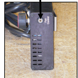
Fan control jacks.
