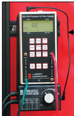
Fan control cable with Blower Door controller.
